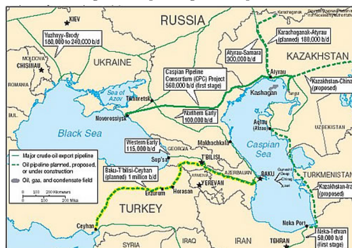
Figure 1: Caspian Region Oil Pipelines
